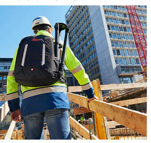
Laser scanning eliminates your team's reliance on antiquated field verification practices and site revisits. With scan-to-BIM, the data can be converted to an accurate Revit model that can be measured and manipulated, allowing you to build the property the owner is expecting. Your model is no longer a representation of design intent, but a digital twin of what was built.
